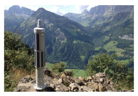
The movement speeds and directions in a glide area in the municipality of Glarus Süd in the Swiss Alps are being monitored over the long term using five autonomous, solar-powered single-frequency GNSS stations.
